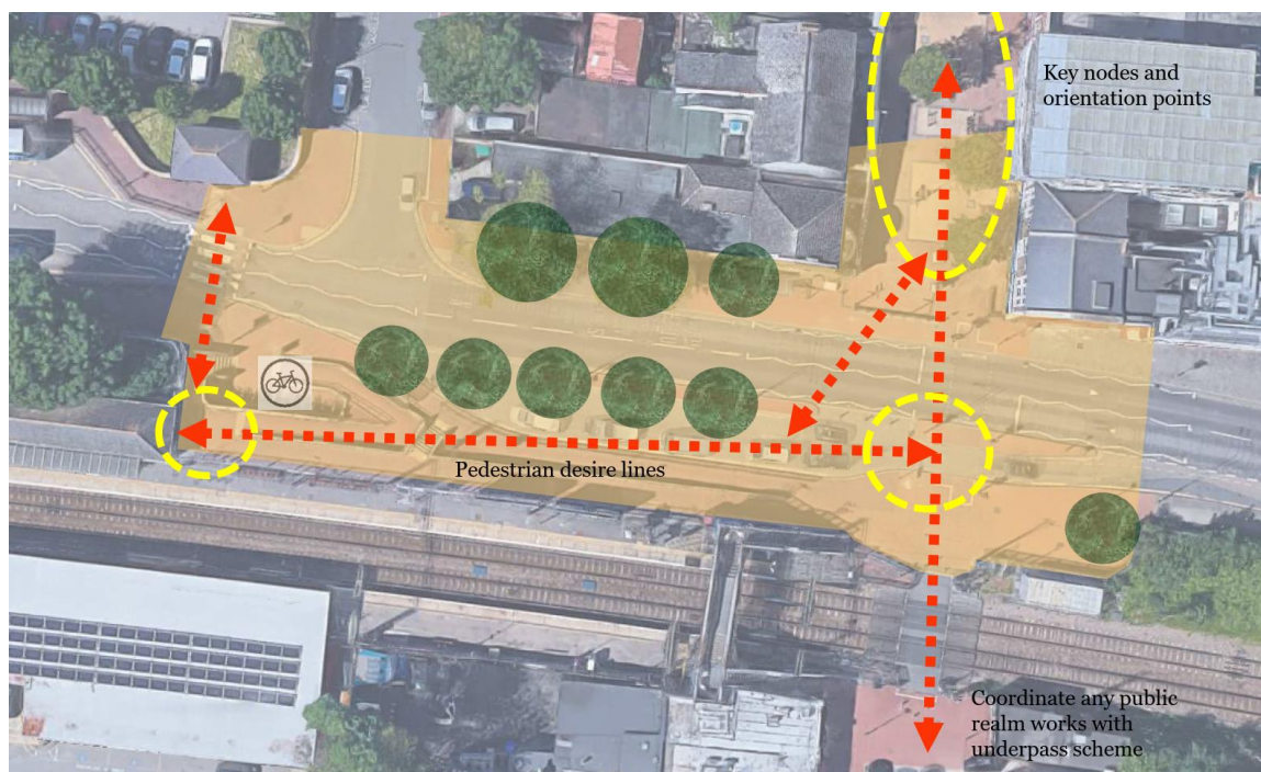
Figure 5-13 Possible Station Square Design
