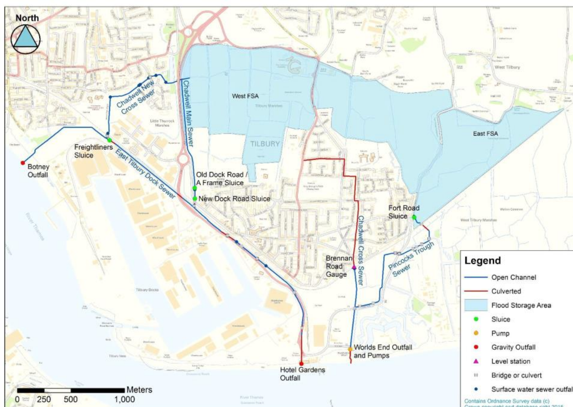
Figure 3-3 Tilbury Integrated Flood Storage Area – Drainage Outfalls
