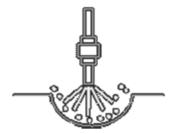
**Stage One:** Using the high volume, low pressure blower to blow all loose debris from the pothole, it is then cleaned and prepared for an effective patch.
