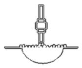
**Stage Four:** After the pothole has been effectively sealed and filled, a light layer of dry aggregate is applied to the patch, preventing the patch from adhering to car tires prior to the emulsion fully curing. The patch is now ready for traffic.
