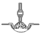
**Stage Three:** Aggregate is introduced into the pothole. The aggregate is mixed with the asphalt emulsion and blown in to the pothole at high velocity.
