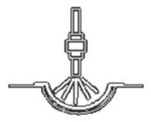
**Stage Two:** The apparatus now coats the pothole with an asphalt emulsion which seals the pothole and prevents further damage from occurring. This is due to the asphalt emulsion providing a waterproof coating, sealing it from encroaching moisture.
