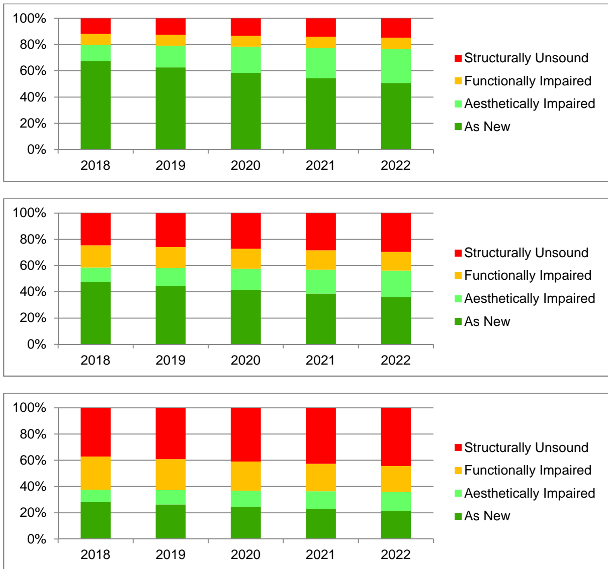
Figure 20 – Best (top), median (middle) and worst (bottom) scenarios derived from FNS results (example surface: bituminous)
