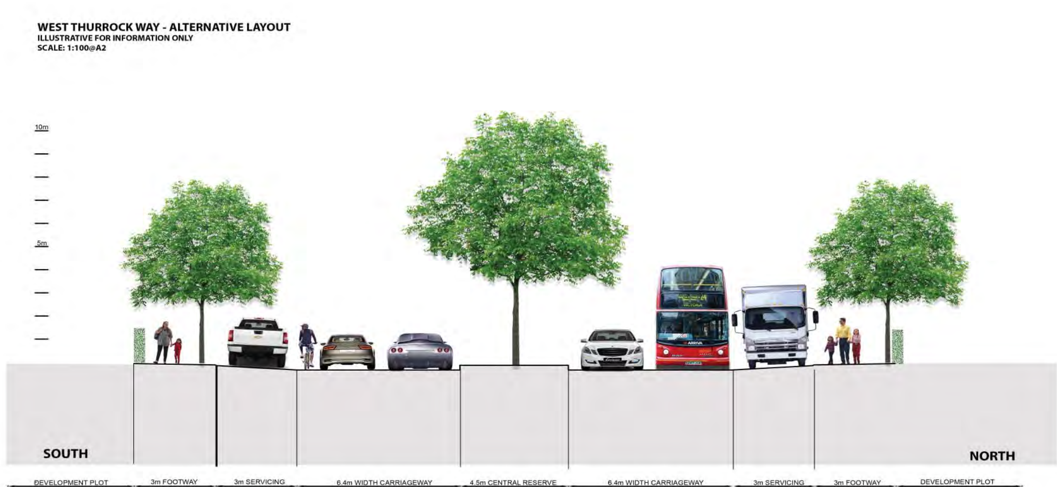
Fig. 44 - Indicative cross section of West Thurrock Way based on future option C(ii) on link 3
