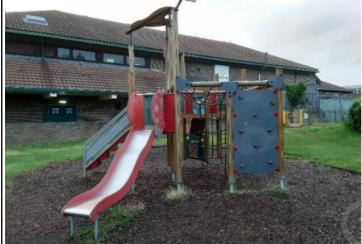
**Finding:** The height of the slide runout is in excess of 350mm and fails the requirements of BS EN 1176: Part 3
