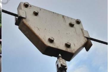
Action: Repair the damaged traveller brake
