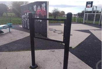
**Finding:** There are no instruction labels provided on the fitness equipment; an instruction label should be provided with each item of equipment in accordance with the requirements of BS EN 16630
