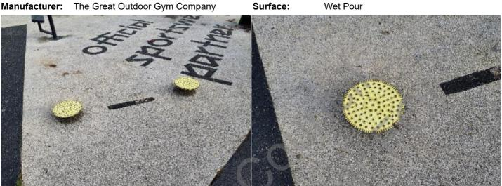
**Finding:** The deflection of the rotating user station exceeds **Action:** Monitor - No remedial work recommended the maximum 105 degrees required by BS EN 16630
